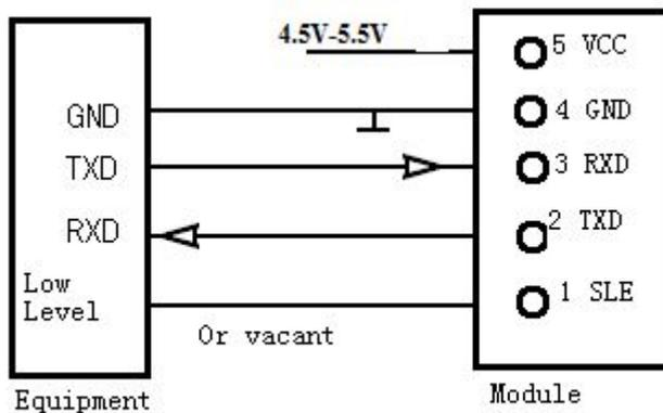
Note: JZX893 did not sleep in the state, the module of the SLE feet must be vacant. In the sleep state when the module must be low, the module can send and receive data.
