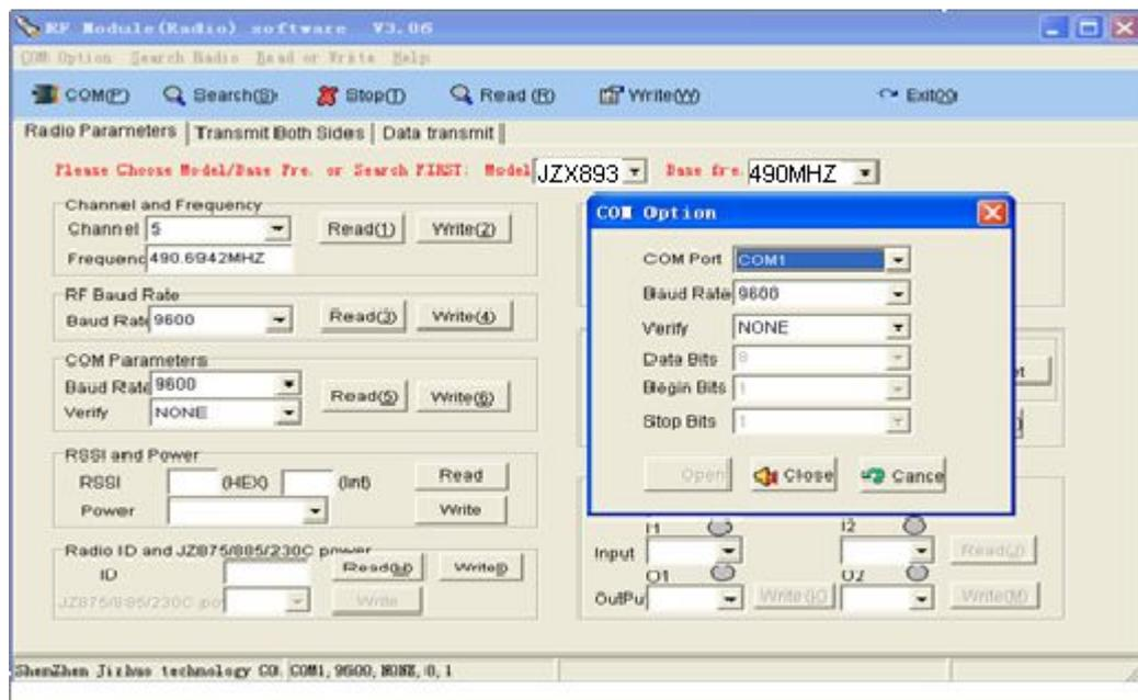
A, between the JZX893 module and connect a PC RS-232 to TTL adapter, and plug in the power, select the serial port used.
