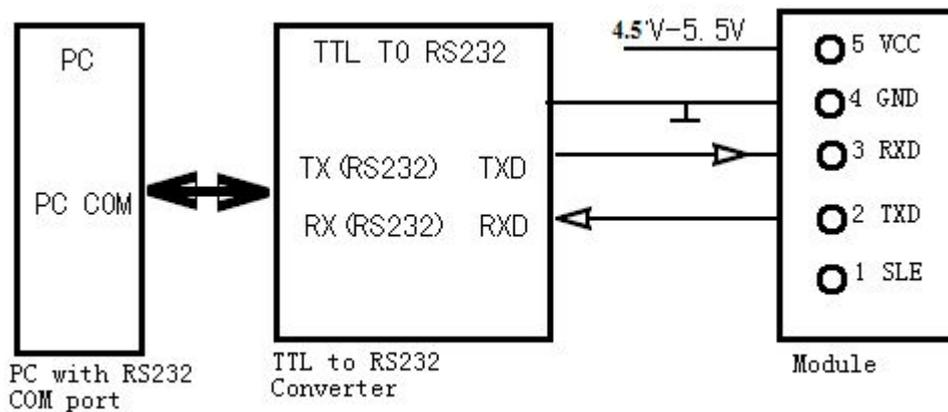
Note: As JZX893 mode TTL interface module, so the PC must be added to connect the TTL to RS232 converter, and converter must supply DC 5V of electricity.
