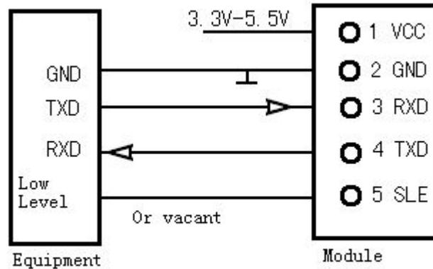
Note: JZX861 did not sleep in the state, the module of the SLE feet must be vacant. In the sleep state when the module must be low, the module can send and receive data.
