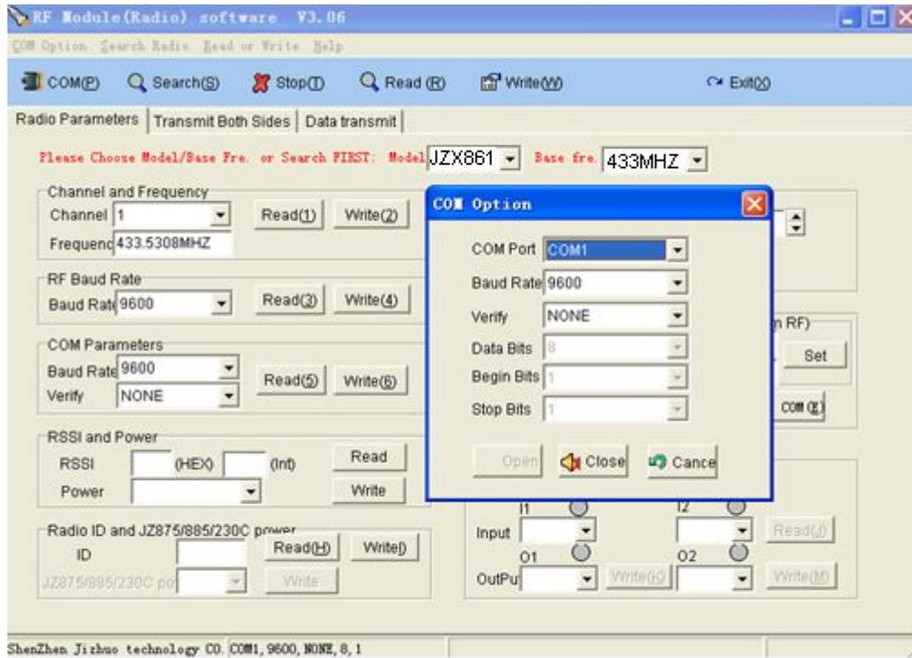
A, between the JZX861 module and connect a PC RS-232 to TTL adapter, and plug in the power, select the serial port used.
