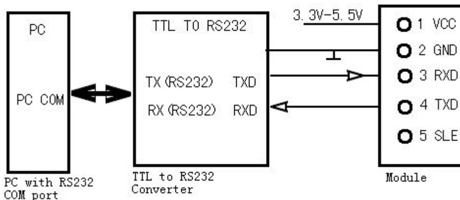
Note: As JZX861 mode TTL interface module, so the PC must be added to connect the TTL to RS232 converter, and converter must supply DC 5V of electricity.
