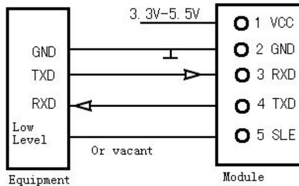
**Note:** JZX863 did not sleep in the state, the module of the SLE feet must be vacant. In the sleep state when the module must be low, the module can send and receive data.
