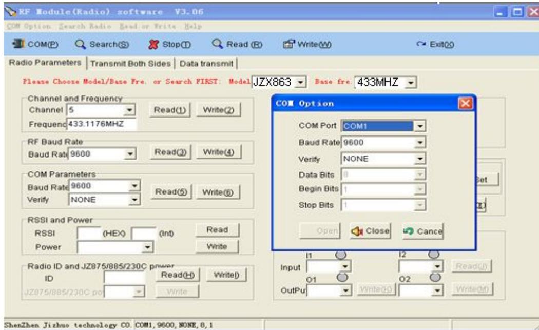
A, between the JZX863 module and connect a PC RS-232 to TTL adapter, and plug in the power, select the serial port used.
