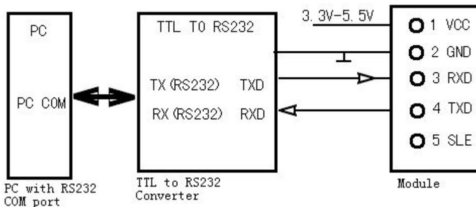
**Note:** As JZX863 mode TTL interface module, so the PC must be added to connect the TTL to RS232 converter, and converter must supply DC 5V of electricity.
