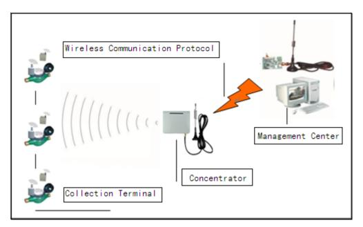
1) Meter reading management center: It composes of the inner meter reading management computer and the background PC management software. It is the core management section of the whole wireless remote meter reading system. It is only the manager of remoting all the wireless meter reading system, but also a bridge to link the marketing management system and remote auto-reading-meter system.
