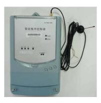
3) collection terminal: also called user terminal. It is user to directly collect the data of usin g. And transmit the data to the centeralized controller by wireless data communication. Coll ecting terminal installed in each building concentrated near the water meter. The location as follows:
